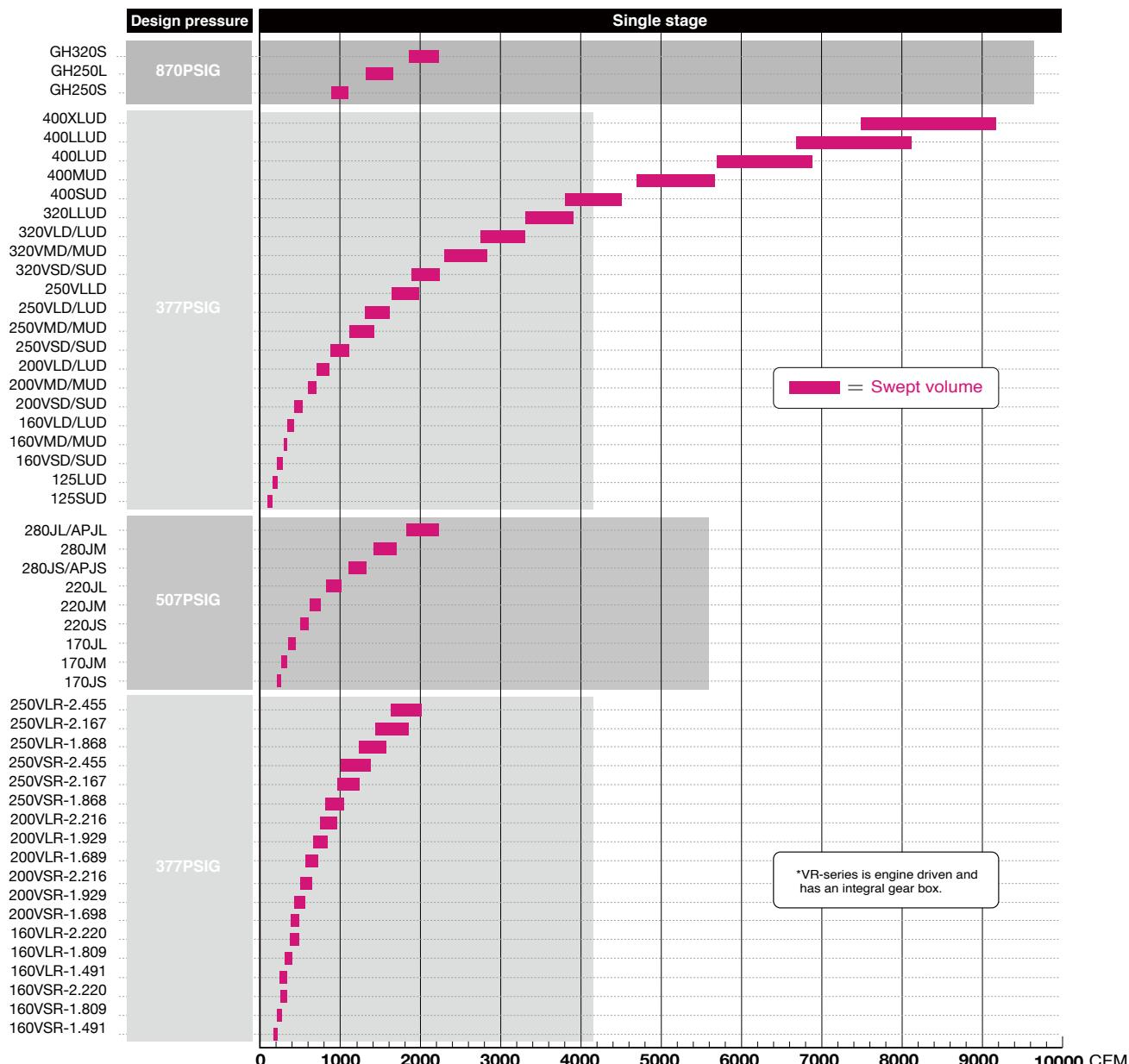
Under the MYCOM brand name, Mayekawa's compressors are in use in industrial refrigeration/freezing, heat pump, and gasmarkets around the world. Leveraging the thermal technology we have fostered through years of experience, we have developed compressors of the highest quality and consistency. And, having focused on prevention of global warming and ozone layer protection from an early stage, we can offer a full lineup of environmentally-friendly compressors that use natural refrigerants.
